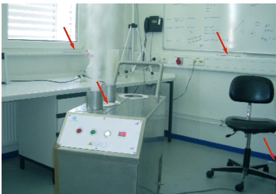
Figure 1: Aerosol generator in operation; the arrows point to the locations at which the exposed germ carriers are visible from this angle within the experimental room.
