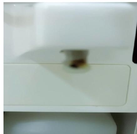
Figure 1: Dispenser type 1 with soiled nozzle .
